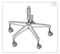
Firmly push casters into base. Insert pneumatic cylinder into base.
