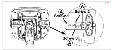
Attach left and right arms using the 3 screws
