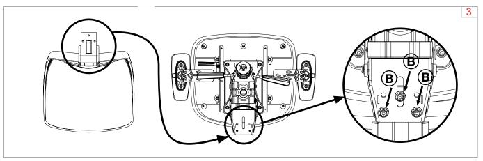
Attach back using the 3(4 for Apt-V) screws provided. (Allen key provided but power driver quicker with screw attachment is quicker) Back should be pulled to rear position before inserting screws. 背もたれを、付属の3本(アプトVは4本) のネジでシートに固定します。
