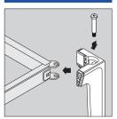
**Cast legs** attach to steel frame with bolts at each corner of the frame.
