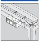
Power strips can attach to underside of any base frame. It can be mounted anywhere along the frame, but must avoid locations that interfere with leg connections.
