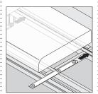
Seat cushions have standard brackets that secure to frame and frame extension without fasteners.
