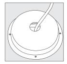
Bottom: Power and data cords exit through hole in the bottom of the caddy.
