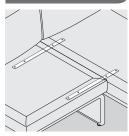
Alignment connector bracket package includes two seat attachment brackets and one screen alignment clip. The alignment connector bracket package is used when permanent connection is needed for L-, U-, and straight configurations of two or more pieces. The screen alignment clip is not needed for any bench connections, only the two seat attachment brackets would be utilized. The alignment connector bracket package should not be used if reconfigurations of the furniture pieces are required.
