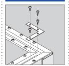
For panels joined in an L-configuration, use two straight lengths of ceiling track, placed perpendicular to each other using a cornice track L bracket.
