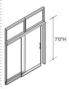
Transom-height slider doors can be specified from 8'0"H to 10'0"H, in one-inch increments. Door height is always 7'. Transom-height varies depending on ceiling height.
