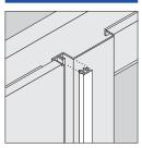
Feature strips, ordered separately, join door frames to panels, posts, adapters, and other components while preventing light and sound leaks. To rearrange doors, feature strips can be removed and reused.
