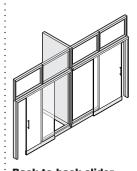
**Back-to-back slider doors** will work with all adapters and posts when slider doors are on the outside of an office.
