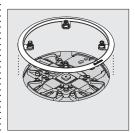
The plastic trim ring is spring loaded to provide a tight fit against the carpet. It provides a simple ramp transition to the 1/2" maximum height of the connector cover and hides any imperfections in the access hole cut in the carpet.
